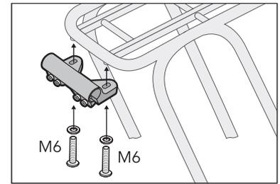
3. Insert the two M6 bolts through the slotted holes of the clamp and screw into the fittings on the underside of the rack. **HAND-TIGHTEN BOLTS SLIGHTLY – CLAMPS STILL NEED TO BE ABLE TO MOVE.**
