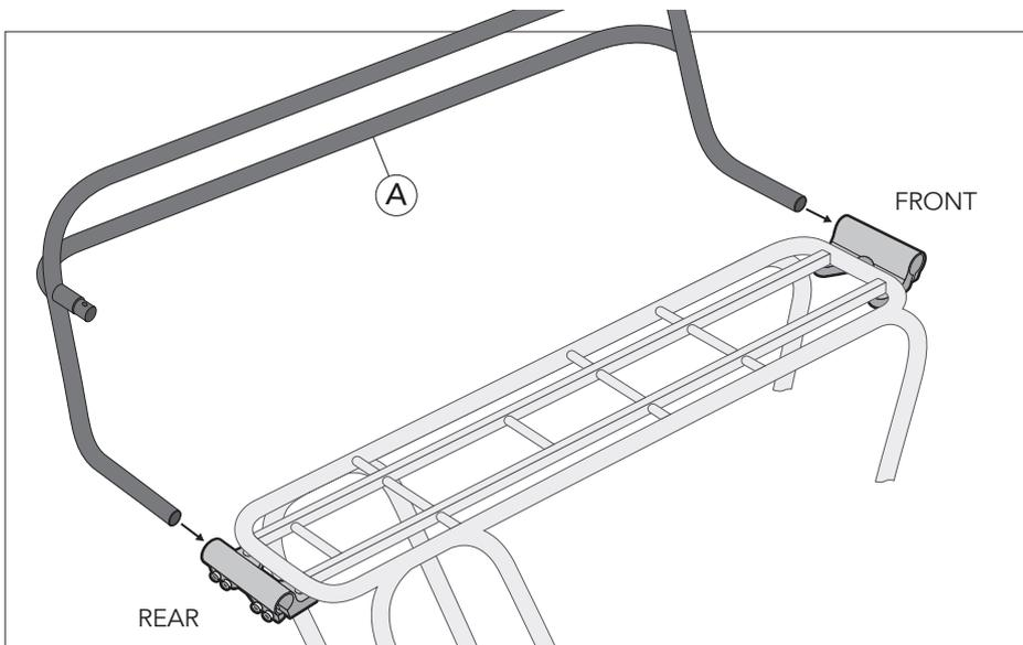
4. Insert both lower ends of left rail (A) from the left side all the way into the center of the clamps until they come to a stop. Loosen clamp bolts as needed for easy insertion. **DO NOT TIGHTEN YET.**
