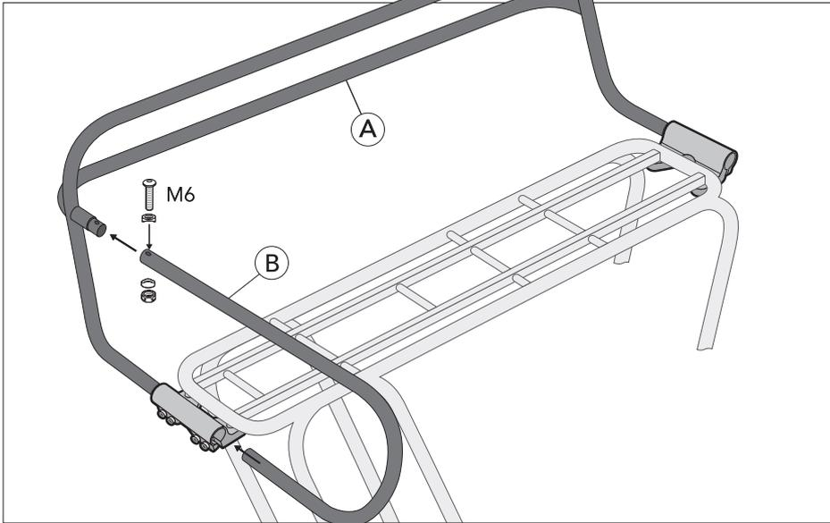
5. Insert the lower end of the rear rail (B) from the right side into the center of the rear clamp until it comes to a stop while connecting the upper end to the left rail (A) as shown. Use M6 bolt, spacers and nut as shown to ensure secure connection between rail (A) and rail (B).
