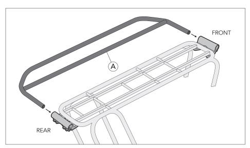
4. Insert both ends of rail (A) from the left side all the way into the center of the clamps until they come to a stop. Loosen clamp bolts as needed for easy insertion. DO NOT TIGHTEN YET.
